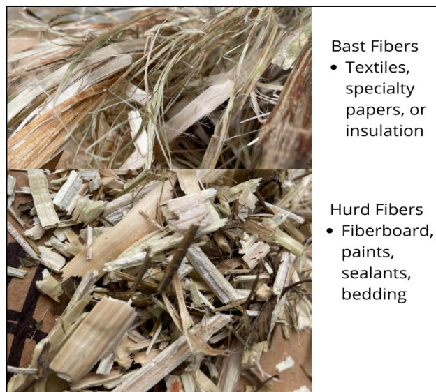
Figure 1. Fiber hemp bast and hurd fibers and different uses of each. Photo Credit Jodie McVane
